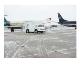
SAFEGRIP is high performance anti-icing and deicing liquid prepared for runways, taxiways and concrete pavements.
